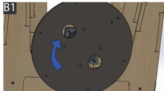
3. After removing the swivel from the chair, use a phillips head screw driver to unscrew the screws holding the round metal base onto the swivel. Use a 1/2 sized wrench to hold the nuts in place so you can remove screws (figure C1).
