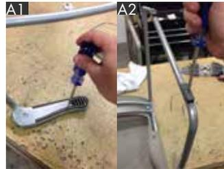
2. Keeping the chair upside down you will notice screws holding both the plastic buffer and the seat to the metal frame. Unscrew these screws.
