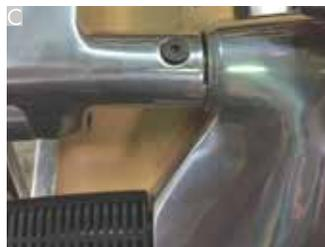
4. Hammer the base off the cylinder by holding the base firmly upside down off the table and hitting the bottom of the cylinder with a mallet. Using moderate force, pull the casters off the base. If stuck, use the mallet.
